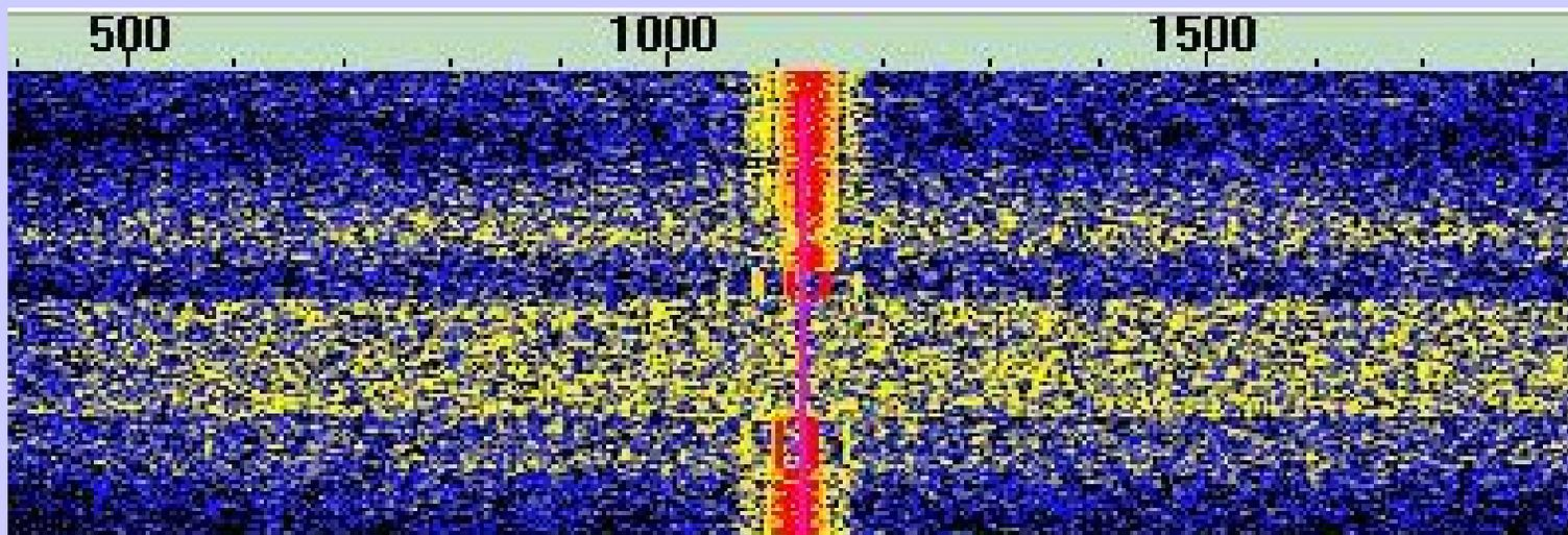
You will notice the slight shift from the two stations signals. Most PSK31/63 software will automatically track slight shifts with the AFC (Automatic Frequency Control) setting. NBEMS/FLDIGI is one of the best in this respect. But AFC is not available with Olivia and MT63, so sound card calibration can be critical.
