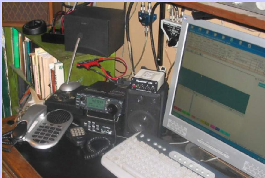
*To start playing around... all you need is an inexpensive computer microphone! Just plug a mic into your sound card mic input and place the mic element somewhere near your radio speaker. Listen and watch your display and practice differentiating the various modes.*
