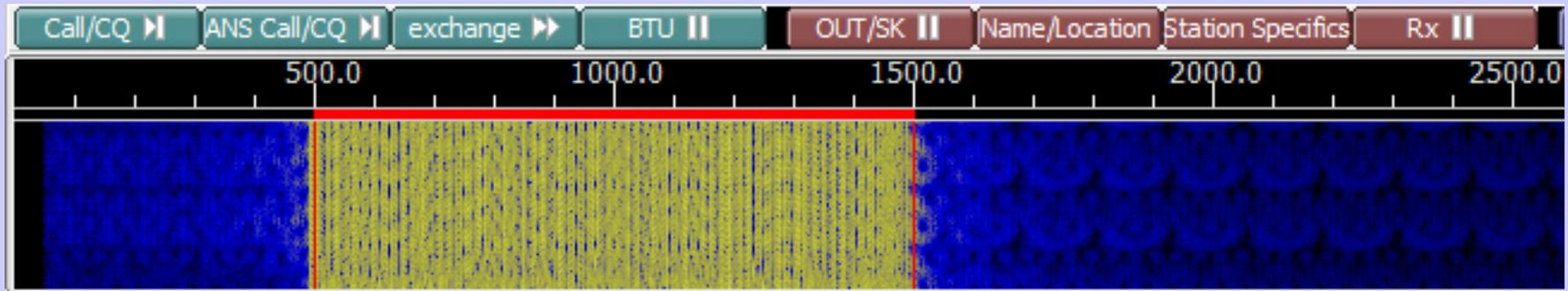
MT63 1k long was chosen for portable, mobile and fixed station operations on HF USB under moderate to good conditions. It is our primary mode for detailed situation reports and database transmissions on HF for the following reasons:
