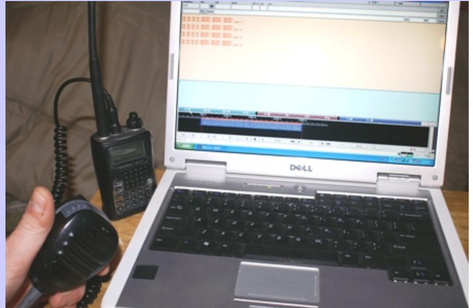
The majority of the wpaNBEMS testing group are using the audio coupling method with great success, weekly. Audio coupling has also been used in the field here in WPA during the Rachel Carson Trail Challenge and during several drills in O'Hara Township.
