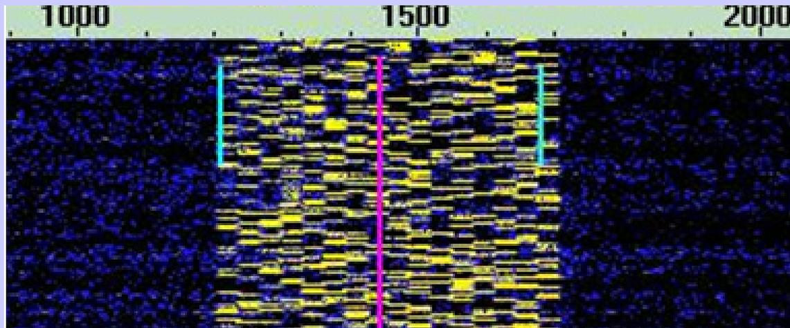
Olivia 16 tones, 500 Hz mode was chosen for use in formal short message handling. Although the mode is relatively slow (about writing speed), it is very accurate, even under extremely poor conditions.
