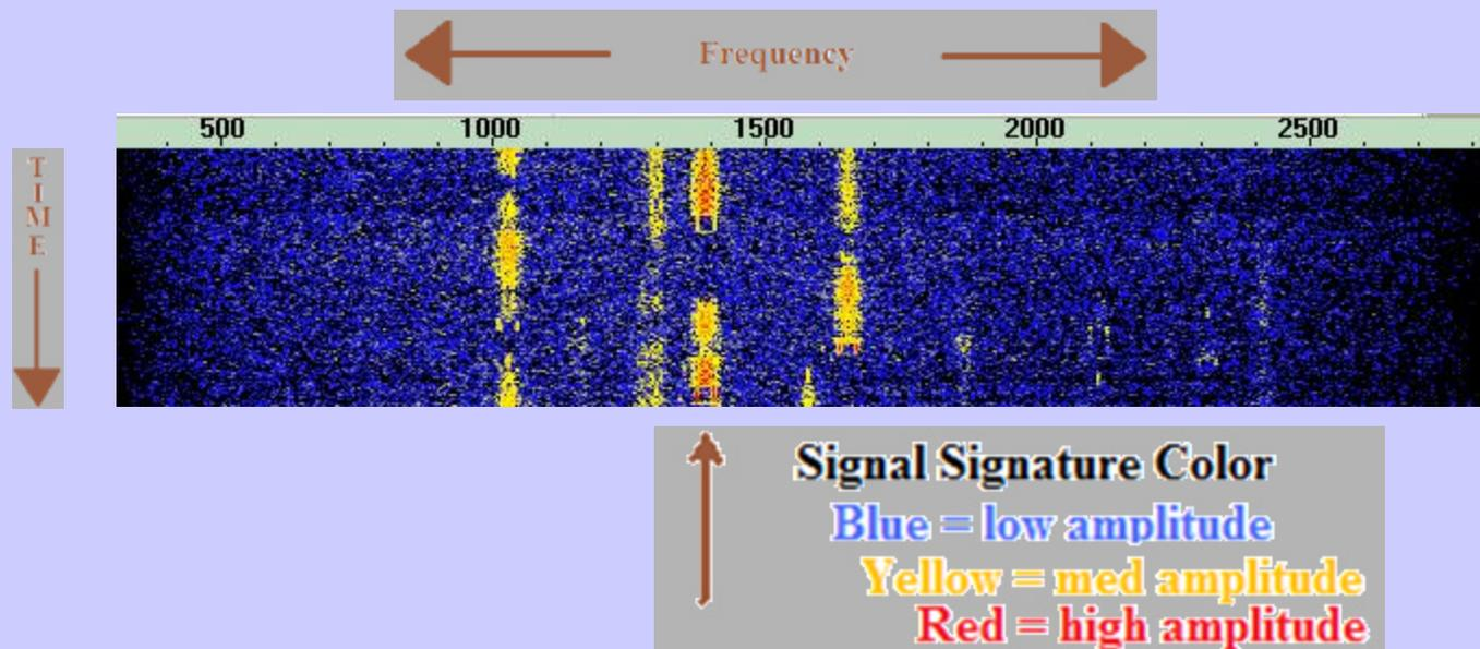
The digital waterfall is a visual representation of time, frequency and amplitude.
