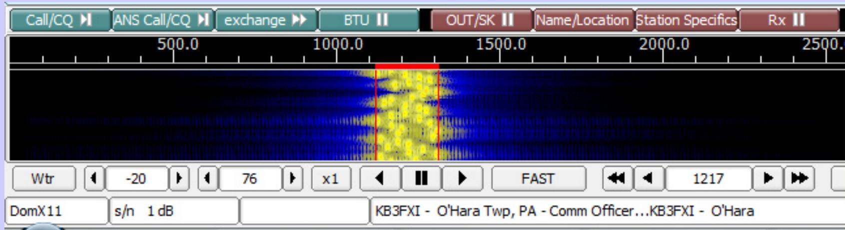
DominoEX11(FEC) was chosen for use in keyboard to keyboard transmissions, assuming that HF conditions are moderate to good. This mode provides a reliable means of sending and receiving short messages. Tuning is not as critical as other modes.
