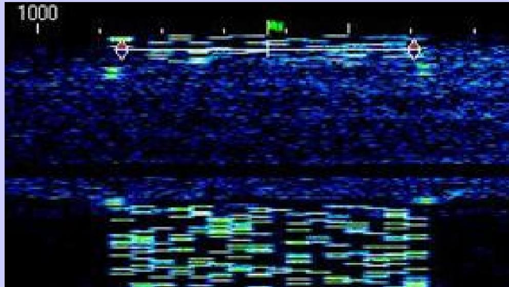
**Our standard is 16/500 but other common Olivia operations are transmitted in 250, 500 and 1000Hz bandwidths. Tuning and sound card calibration are critical on this mode, but Olivia is capable of maintaining near 100% copy under extremely adverse conditions.**
