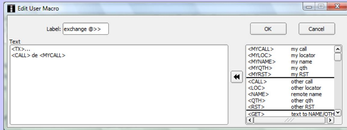
A right-click on the macro buttons on most programs brings up an editing function that allows you to change the macro text or functions. The macros allow the operator, for example, to send preformatted text and information with a single mouse click. The macros also automate transmit and receive functions from the computer to the transceiver.
