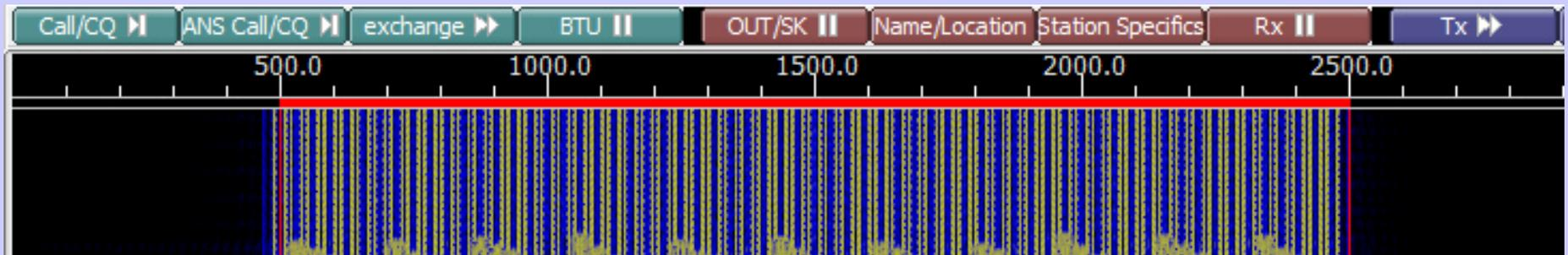
MT63 2k long was chosen for local portable, mobile and fixed station operations on FM channels (repeater or simplex). It is extremely well suited for detailed situation reports and database transmissions for the following reasons:
