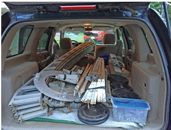
Complete set of components for the 14 foot communications dish loaded in the back of Steve Crusse's van right before we headed back to Pennsylvania from Virginia (this included 400 pounds of barbell weights that are going to be used as counterweights for the dish).
