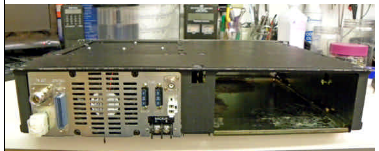
Above - The rear of the repeater unit after a little cleaning & polishing. Below - The completed, reassembled repeater after all cleaning was done. All that should have to be done is reprogramming to our frequency and some testing.
