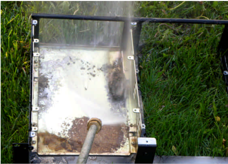
Utilizing a high pressure power washer, Skip took the repeater outside and washed out the accessory bay.
