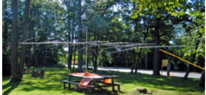
Shown here is our HyGain TH-7DX Triband Beam ready to go up. This antenna was donated to the club by Jim Walsh, K3JIM. I have never seen a HF beam with as nice a set of SWR curves as this one!
