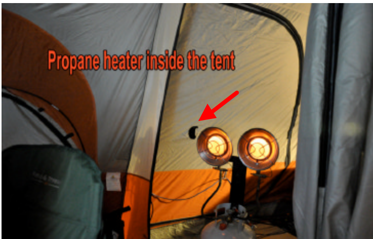
Heat was provided by a propane heater. While this kind of heater does not emit harmful quantities of Carbon Monoxide, it could possibly deplete the area of Oxygen. In our case however, the tent was extremely well vented so this wasn't an issue. We did worry about it being blown over because of the tent moving in strong winds. At one point, the wind blew so hard that the side of the tent touched the back of the heater and this melted a hole in the side (see arrow).
