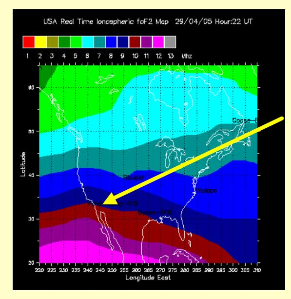
Here our critical frequency is close to 10 MHz. This was several <u>years before</u> the bottom of the solar cycle.
